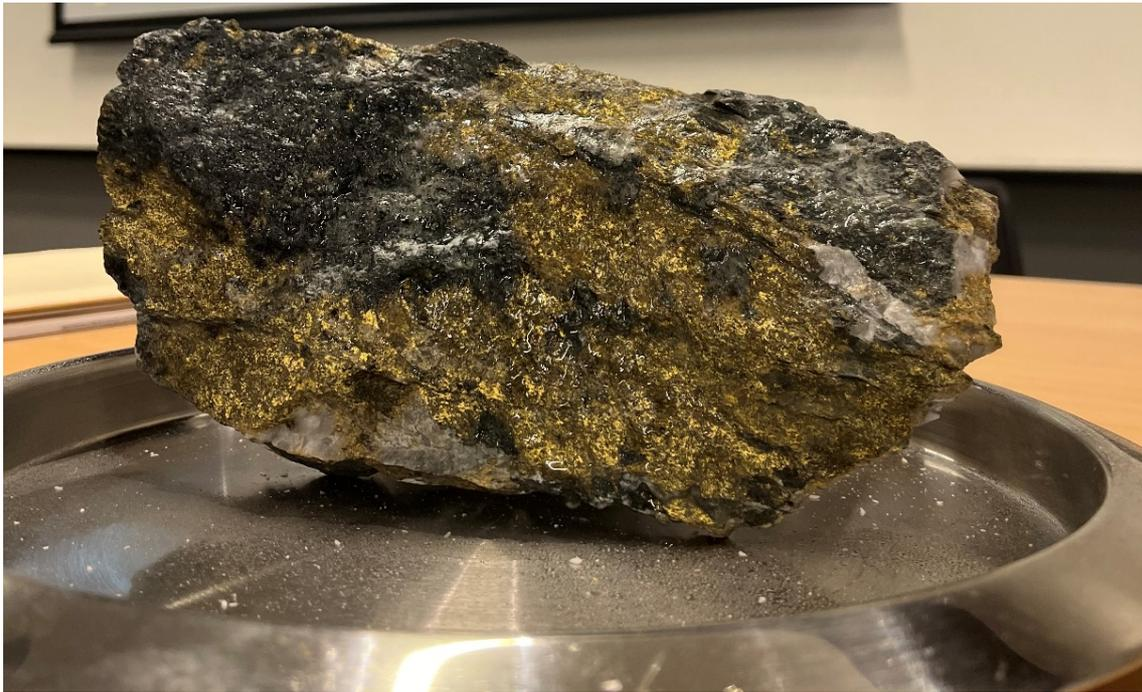
**Figure 4 – Grab Sample from Nightfall Lode (visible gold evident).**
