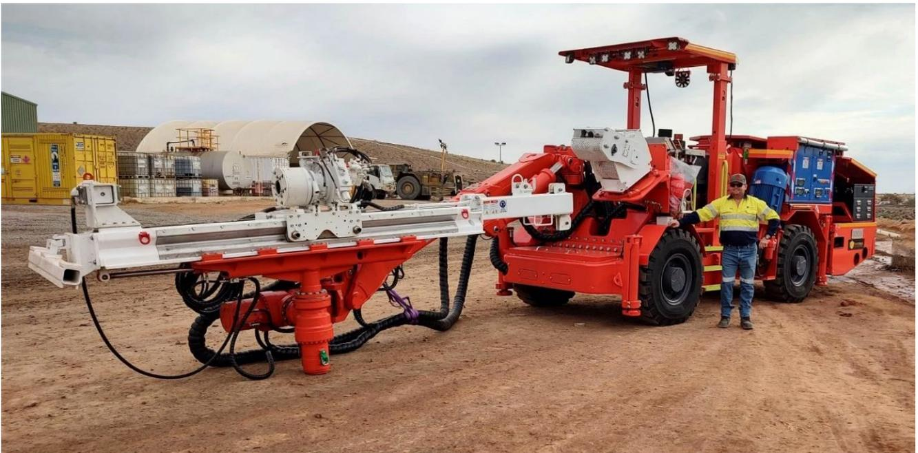
Figure 14: Westgold underground diamond drill rig.
