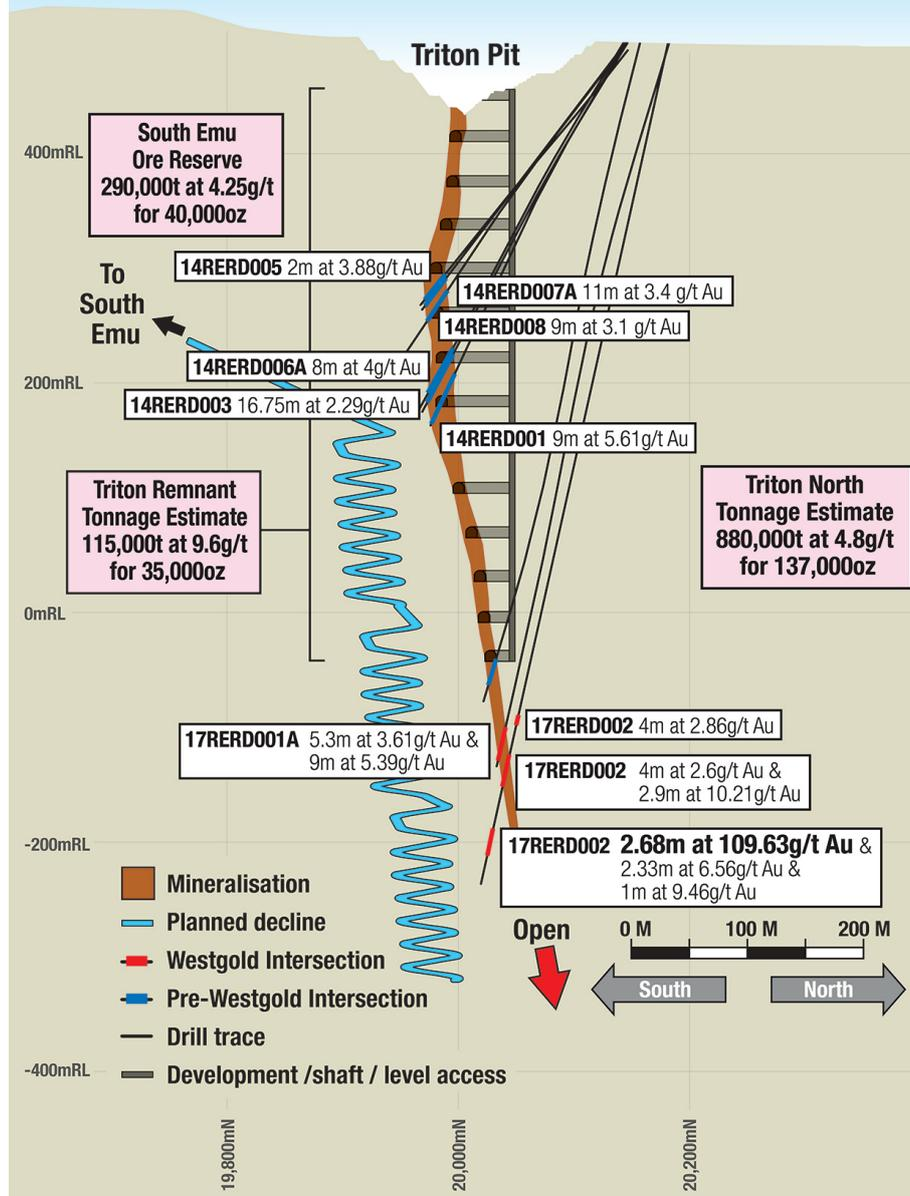
Figure 2: Triton - South Emu schematic cross-section 40,300mN (Reedy Local Grid).
