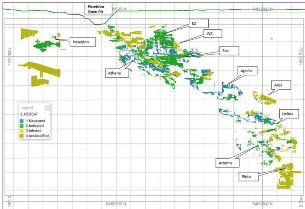
**Figure 14-8 Trident block model coloured by resource classification – long-section looking west – Source: Westgold.**
