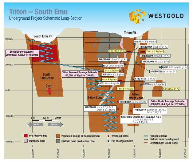
Figure 1: Triton - South Emu project schematic long-section.
