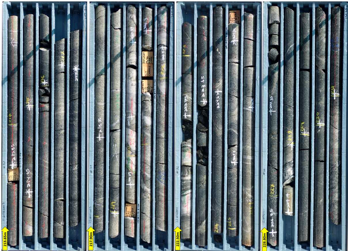
Figure 13 – Sovereign Target Drill Hole 22GFRD003 (213-231m) (Assays Pending) Showing Intersected Quartz Reef and Alteration System
