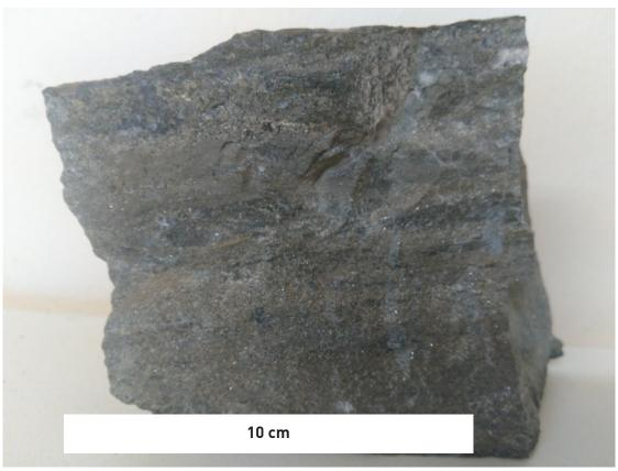
Figure1: Pyrite-sphalerite massive sulphide.
