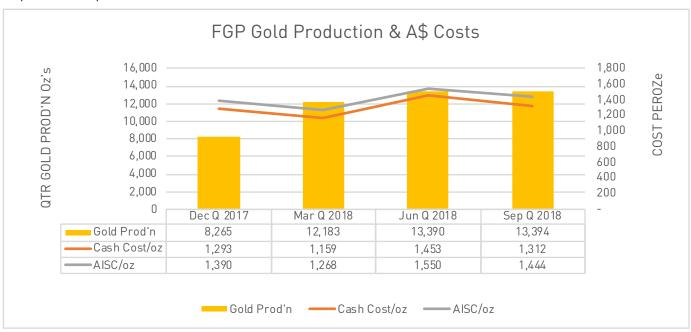
In the past twelve months the Fortnum Processing Plant processed approximately 868,000 tonnes and has struggled to achieve the expected one million tonnes per annum. Modelling of planned ore sources in the coming year suggests that a realistic throughput target is 105 -110 tph or 850 - 900,000 tonnes per annum. Activity levels at the various operations have been re-scheduled for this new target.
