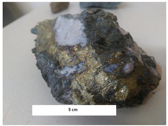
Figure 3: Quartz-chalcopyrite-bornite vein
