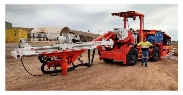
Figure 14: Westgold underground diamond drill rig.
